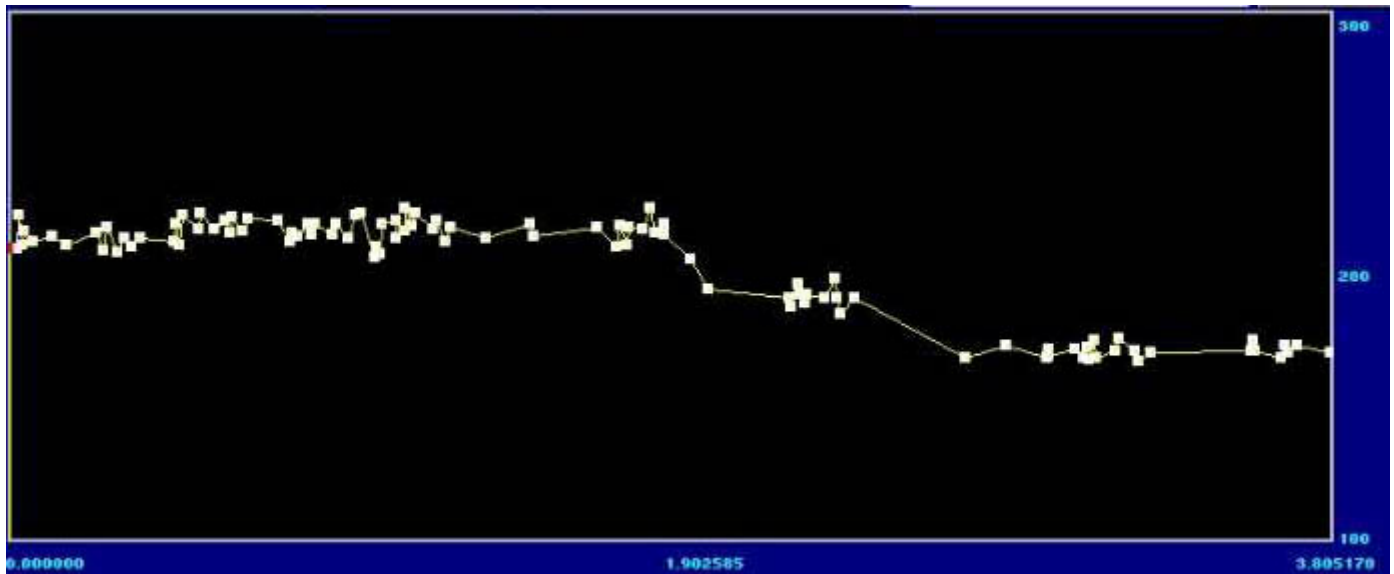
Breakpoint file of extracted pitch from three notes (A-G-F) of sung plainchant.
