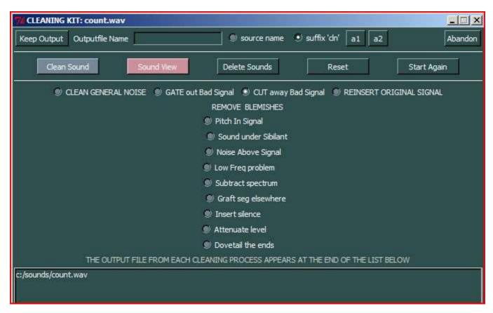
The way these functions relate to the SPECNU programs is hidden to the user, as the *Sound Loom* Cleaning Kit builds the SPECNU functionality into a much broader context. The input to the Cleaning Kit is a normal soundfile, not an analysis file, and when a selection is made and the CLEAN button is activated, new dialogues appear which enable you to enter data and complete the processing.
