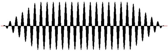
*GrainMill* transforms a sound by cutting it into small pieces, called **grains**, then reassembling the grains to reconstruct a new sound. If we simply cut a sound into chunks, then rejoin them end-to-end in the same order, we will end up with the sound you started with! To transform the sound, we need to reassemble the grains in a new way.
